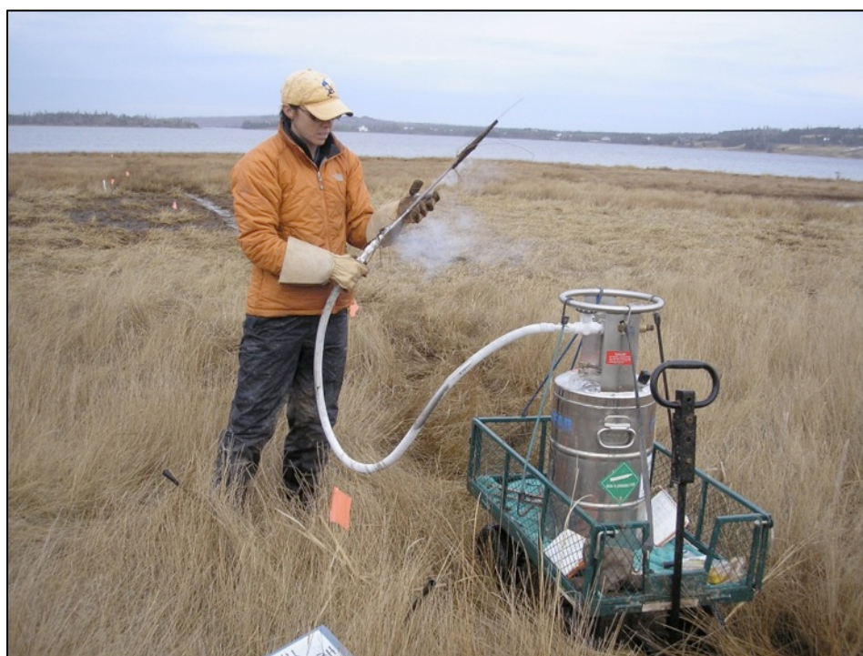
Figure 12 Marker horizon sampling with the cryogenic corer at LT-R. Photograph taken by B. Lemieux, December 2011.
