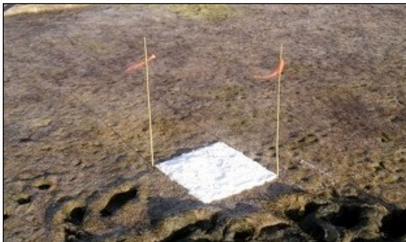
Figure 11 Example of a feldspar clay marker horizon. This is one of the markers established in 2005 at the Walton River Salt Marsh Restoration site. Photograph by T. Bowron, 2005.
